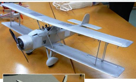
**Top:** Keith Trillo's Stardust Special E Rubber model, showing the tubular balsa rolled fuselage.
